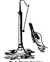
Fig. 2. Electric Repulsion. bring the rod once more near, you notice that the ball is strongly repelled. (Fig. 2.)
